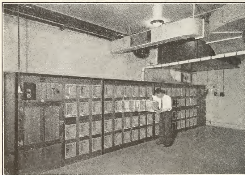
FIGURE 16.—Special battery-brooder room with individual compartments, used in conducting nutrition experiments in which a feed-consumption record of each chick is desired.
